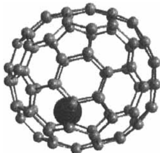
FIGURE 1 The endohedral molecular structure of \text{La}@\text{C}_{82} .
